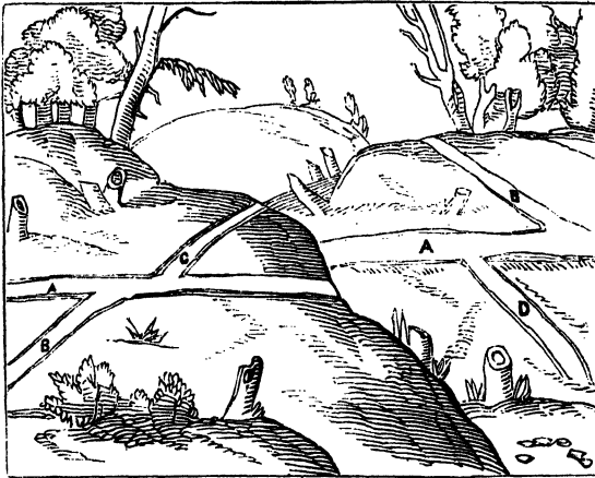
Fig. 161. A. chief vein. B. Intersecting or cross vein. C. The other part of B, removed from its natural position (rapta). The further removal and alteration of the original position and continuity of the vein is shown to the right at D A B. (Agricola.)
